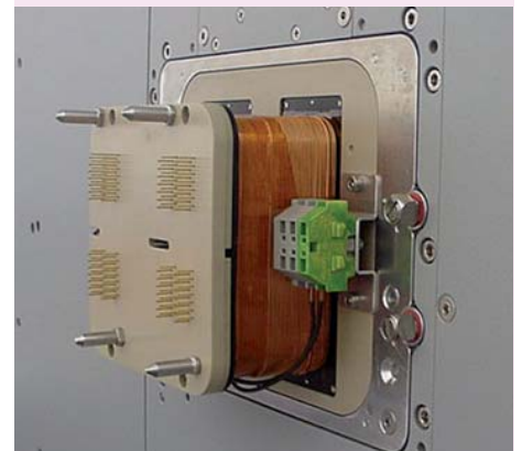
Hall contactor with coil
