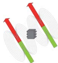
Hall principle: Device is moved into a magnetic field
