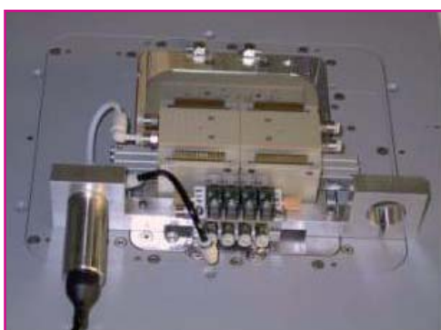
Pressure Contactor (view from tester)
