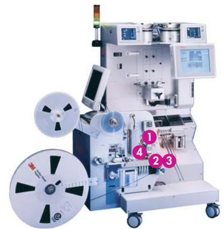
SO2000 with Rasco VisionSystem, Bowl Input, Tape&Reel Output
